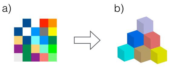
Figure 7. Examples of voxels deleting: simplified view of the model section and two tools with different penetrative tips (a), simplified view of the model section after deleting some voxels (b) (Adapted from [Wyleżoł, 2013])
