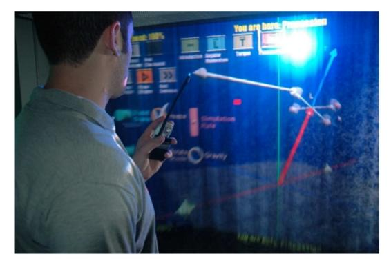
Figure 14. The 3D physics tutorial relied partially on the FogScreen, enabling direct interaction with the objects, e.g., to pull force vectors unobtrusively also through the screen
