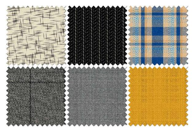
*Figure 3. Examples of CAD simulation for textile –Jacquard weaving (it produced on a special loom, are characterized by complex woven-in designs, often with large design repeats)*
