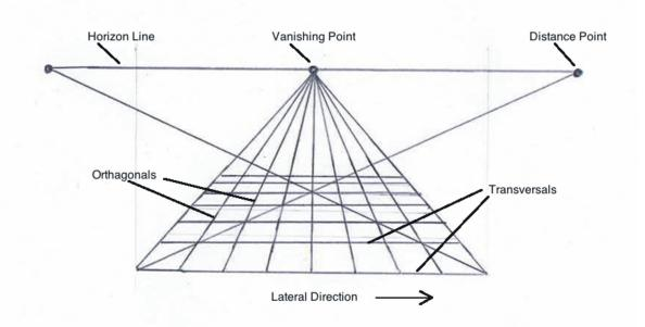
Figure 1. Linear Perspective Construction
