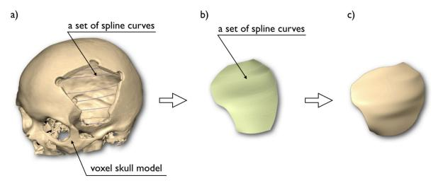
Figure 20. The first stages of the implant modeling process: a) view of the added spline curves, b) surface patch, c) voxel form of the surface path
