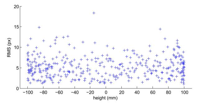
Figure 9. Evaluation of the effects on the reprojection error of different heights of the virtual marker
