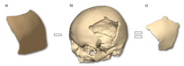
Figure 24. The Boolean subtraction (Adapted from [Wyleżoł, 2013])
