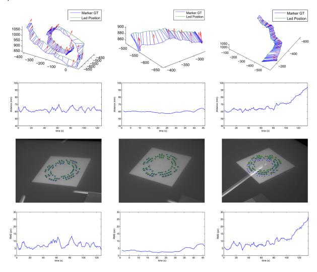
Figure 7. Evaluation of the accuracy in the pose estimation and positional error commited on the image plane
