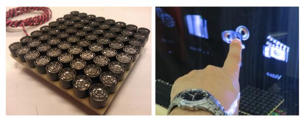
Figure 13. (a) the transducer side of the self-contained ultrasonic tactile module. (b) a prototype of the tactile mid-air display. The array of ultrasonic transducers can be seen behind the fogscreen.
