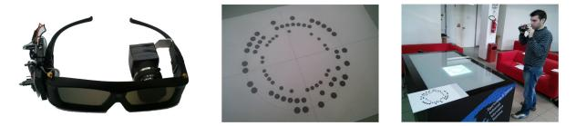
Figure 6. The modified glasses and the fiducial marker used for testing purposes
