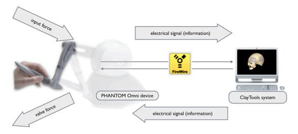
Figure 5. Haptic modeling system – main elements, connections and direction of signals flow
