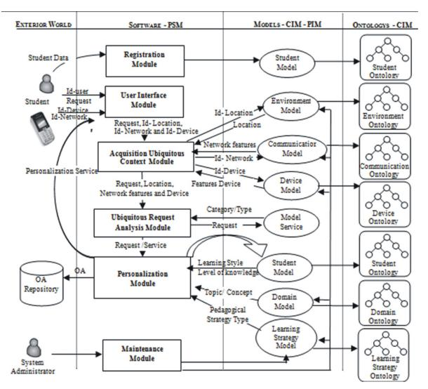
*Figure 7. The Ontological Models-based Architecture for Ubiquitous Learning Application (Durán et al., 2014b)*
