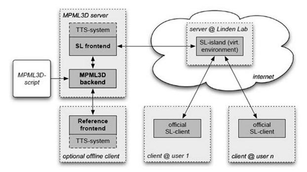
*Figure 4. Overview of the system architecture with the different components distributed over several servers, (Ullrich, S., Prendinger, H., & Ishizuka, M., 2008)*
